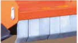
SAFETY BOARDS Plates placed in front of the chassis to prevent safety problems while the machine is running.
